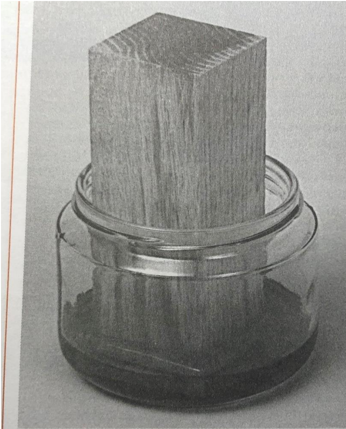
Photo 4-1: Penetration occurs by capillary action. The linseed oil in the jar has risen through the oak and is coming out the top. Deep penetration is achieved by keeping the surface of the wood wet for an extended period of time.
